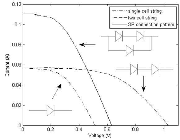
Fig. 2 I-V characteristics of: a separate PV cell, a series connection of two cells in a string, and connection of a two-cell series string in parallel to a single cell. [13, Figure 13]
