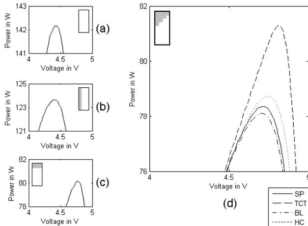
Fig. 3 P-V characteristics of different connection patterns of a 9x4 cell photovoltaic panel under varying shading, i.e. no shade (a), vertical shade (b) horizontal shade (c) and diagonal shade (d). [13, Figure 15 & 16]
