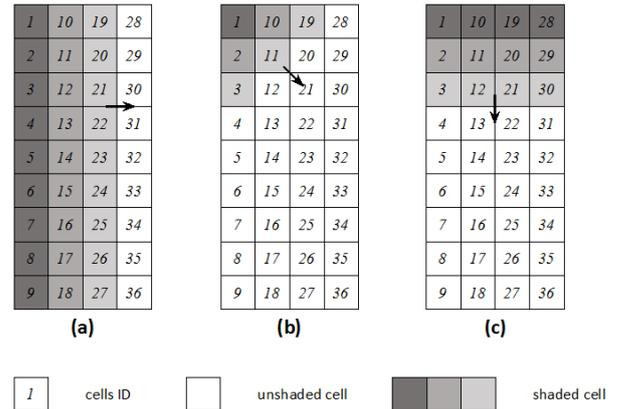
Fig. 8 Progressive shading patterns of the simulated PV panel.
