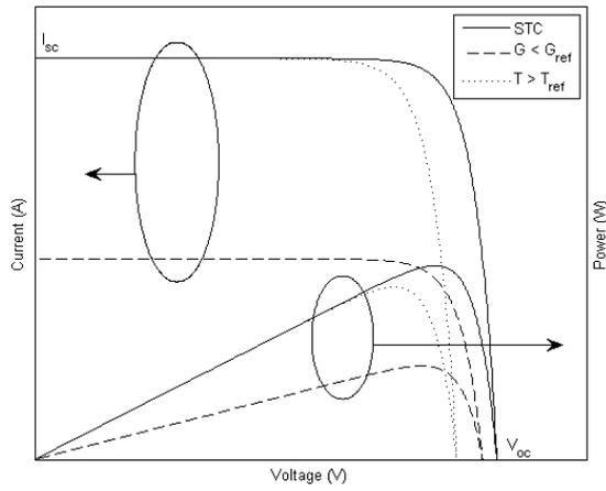
Fig. 1 I-V and P-V characteristics of a typical photovoltaic panel under the influence of different irradiance and temperature values.
