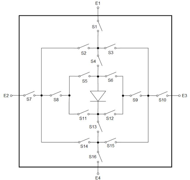
Fig. 5 Electrical schematic of a cell block in the proposed PV panel design.
