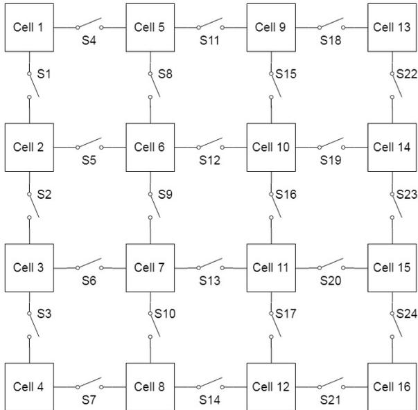
Fig. 4 Possibility of electrical connections of the cell blocks in the proposed PV panel.
