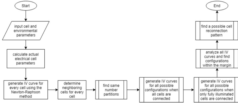
Fig. 6 General flowchart of the algorithm
