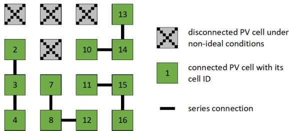
Fig. 7 Result for the reconnection of the test panel.
